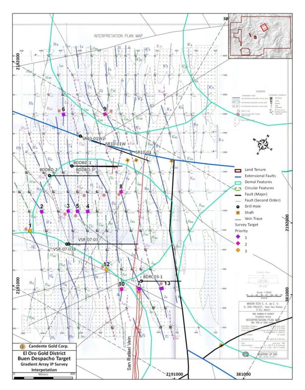
Figure 6.10: Teck 1996 Quantec Gradient TIP Buen Despacho Survey (Priority Targets)
