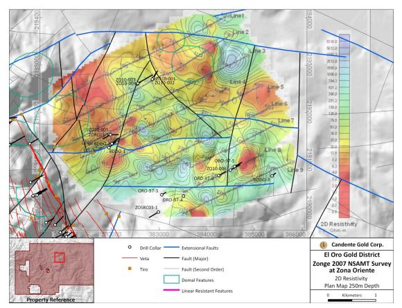
Figure 6.15: Candente's 2007 NSAMT survey showing 2D resistivity at Oriente
