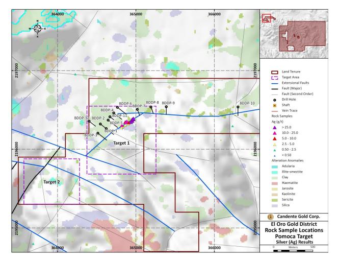
Figure 6.33: Pomoca Vein System Compilation (drilling, alteration, faults and silver)
