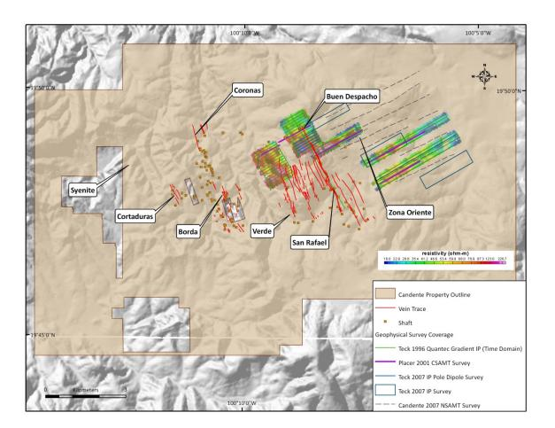
Figure 6.8: Results of the Teck 1996 Quantec Gradient TIP Survey (Resistivity)
