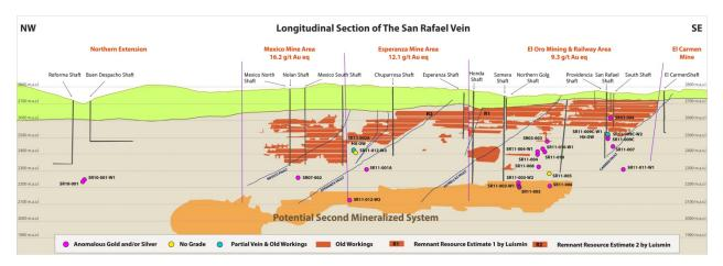
Figure 6.22 San Rafael Schematic Long Section (projected locations of workings, shafts, faults, drill holes)
