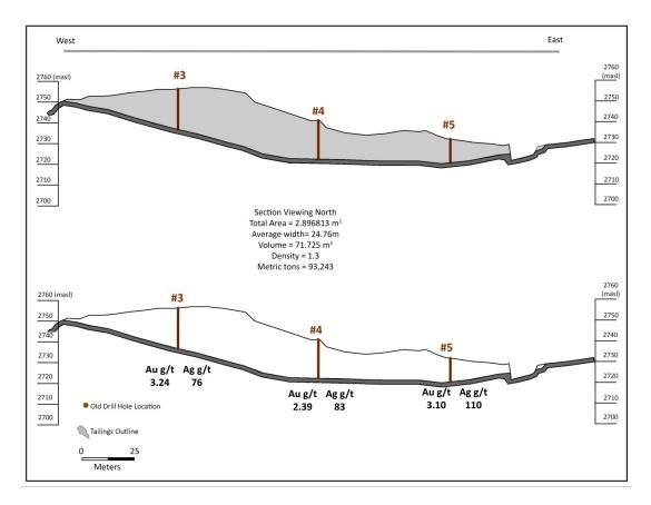
Figure 6.21: Section #3 Showing the Locations of Holes #3, #4 and #5 by Luismin 1990
