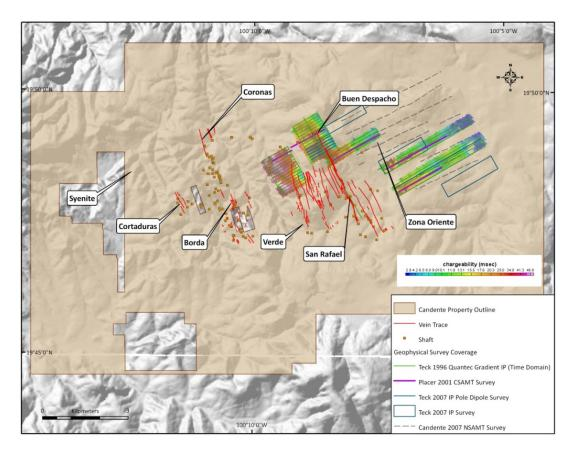
Figure 6.7: Results of the Teck 1996 Quantec Gradient TIP Survey (Chargeability)
