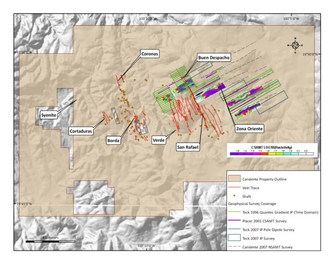
Figure 6.11: Placer 2001 CSAMT Log 10-Resistivity Survey Results
