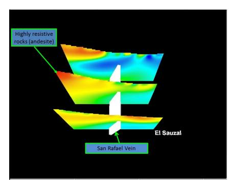
Figure 6.13: Placer 2001 Pole-Dipole IP (looking north) Resistivity
