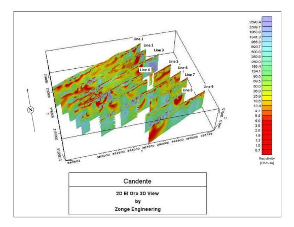
Figure 6.16: Candente's 2007 NSAMT survey showing 2D resistivity sections at Oriente
