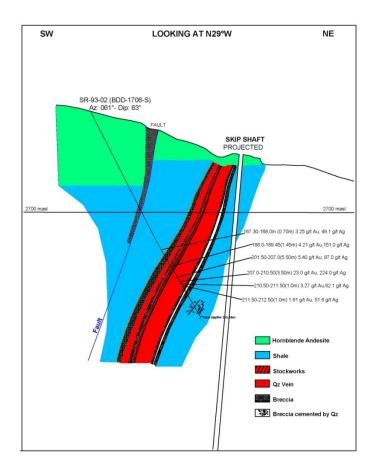
Figure 6.24: San Rafael El Oro Mining & Railway Mine remnant mineralization (Drill Hole SR-93-02)
